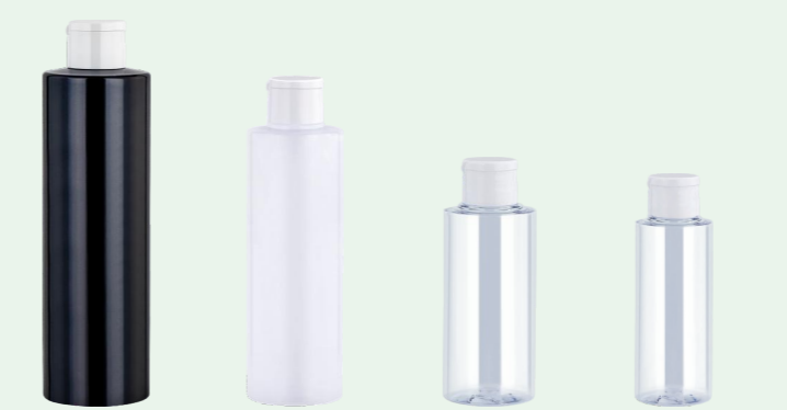
0336-280PET Neck (瓶口): 24mm/410 Capacity (容量): 280ml Size (尺寸) (∅直径xG高): ∅50.7x175.5mm 0408-200PET Neck (瓶口): 24mm/410 Capacity (容量): 200ml Size (尺寸) (∅直径xH高): ∅47.5x155.5mm 0020-150PET Neck (瓶口): 24mm/410 Capacity (容量): 150ml Size (尺寸) (∅直径xH高): ∅46.8x117.5mm 0475-80PET Neck (瓶口): 20mm/410 Capacity (容量): 80ml Size (尺寸) (∅直径xH高): ∅37x102.5mm
